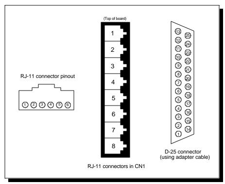
Figure 21 --- ESC-100M Output Connectors
